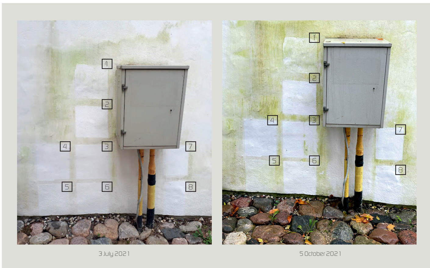
Figure 3: Demo object (the northern wall of St. John's Church) after four and seven months' exposure.
